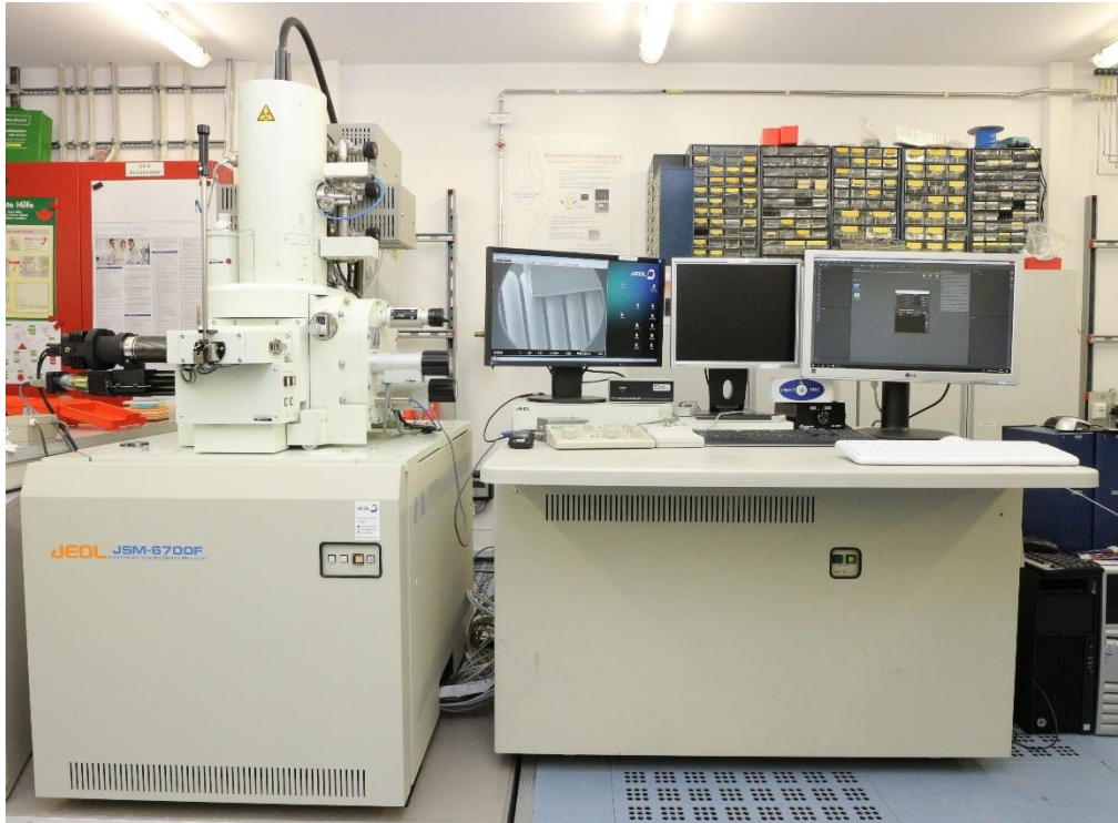
Figure 23. A JSM-6700F (JEOL) scanning electron microscope.
