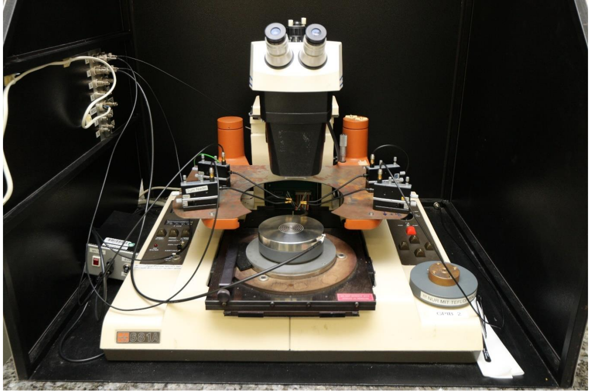
Figure 24. Electrical measurement setup consisting of four micromanipulators with fine needle probes, a metallic vacuum chuck on the motorised stage for wafer sample mounting and an optical microscope.
