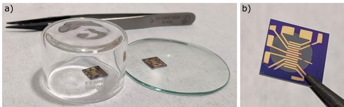
Figure 56. a) S1 and S2 are individually protected by a glass cover over night. b) S1 with a stain left by the dried HEPES buffer droplet after 17 h in atmosphere.
