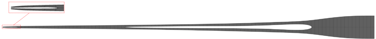
Fig. 22. Design of web A after simplified topology optimization. Zoom on the detail at the end of the blade.
