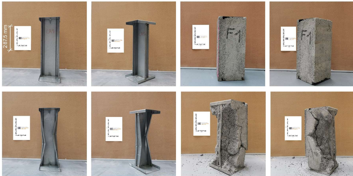
Figure 8. Comparison of test specimens for the composite system. On the left: plain steel profiles connected to horizontal U-profiles at the top and bottom by spot welding. On the right: identical steel profiles embedded in the LAC+. Compression tests for sheet steel profiles ( left ) versus composite specimens ( right ) before ( top ) and after ( bottom ) the test.
