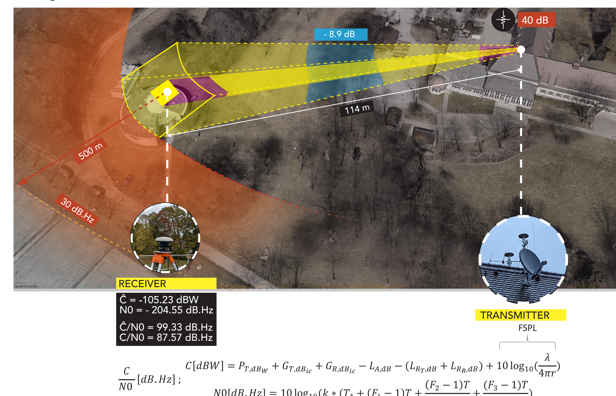
Figure 4: Link budget calculation over the r=114 meters trans-receiver test bed. The estimated direct line-of-sight C/N_0 of 99.33 dB.Hz is validated against the measured C/N_0 of 87.57 dB.Hz, considering an estimated signal attenuation of -8.9 dB due to the canopy. The residual value of 2.86 dB is attributed to the empirically chosen transmitter ( G_{T,AB} ) and receiver antenna gains ( G_{R,AB} ) as well as partially measured (%) transmitter cable losses ( L_{R,T,AB} ), and empirically chosen atmospheric and rain loss ( L_{A,AB} ) terms.
