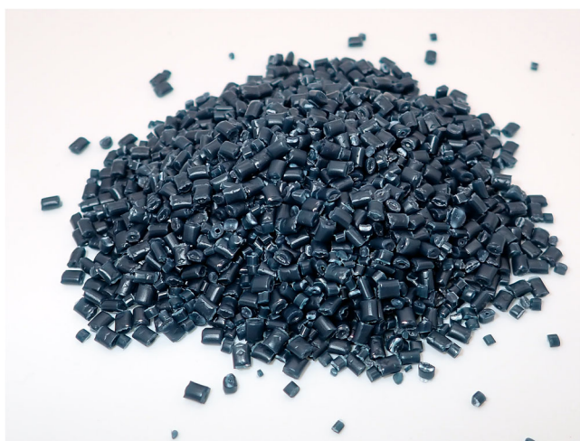
FIGURE 4 Recycled granulate after processing with the twin screw extruder.
