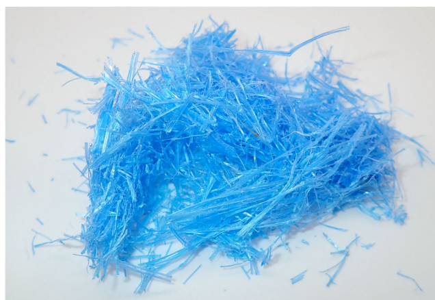
FIGURE 2 Wool-like granulate after shredding of the binding twine.
