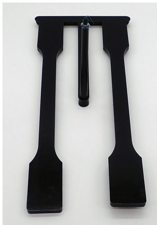
FIGURE 5 Produced tensile test specimen from recycled polypropylene with gate.
