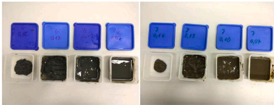
Fig. 5. Gandersum (G) and Jemgum (J) silt samples with the volumetric solid fractions \phi_s = 0.16, 0.13, 0.10 and 0.07 .
