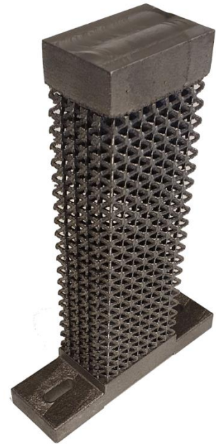
Figure 6.3: ITS thermal lattice specimen without structural double walls to validate the conductive heat
