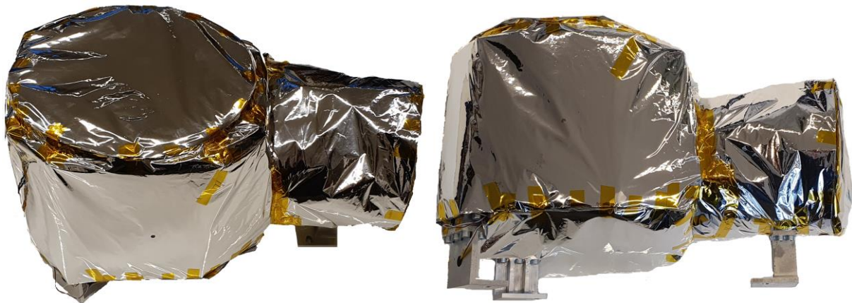
Figure 7.7: ITS demonstrator thermal test setup with accommodated kapton surface heaters, thermocouples and wrapped in MLI. The additive manufactured demonstrator is mounted on aluminium GSE adapter [WIL-23]
