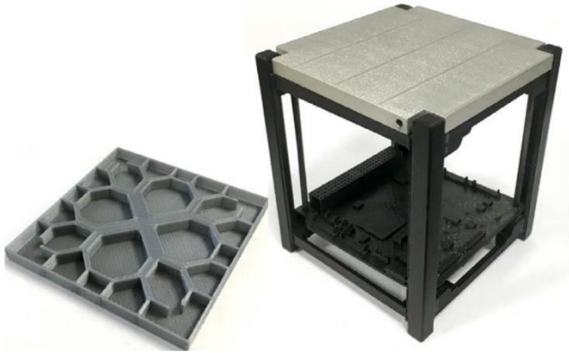
Figure 2.4: PCM panel with an additive manufactured aluminium casing and integrated heat transfer structure for the thermal stability control of a CubeSat [ISA-17]
