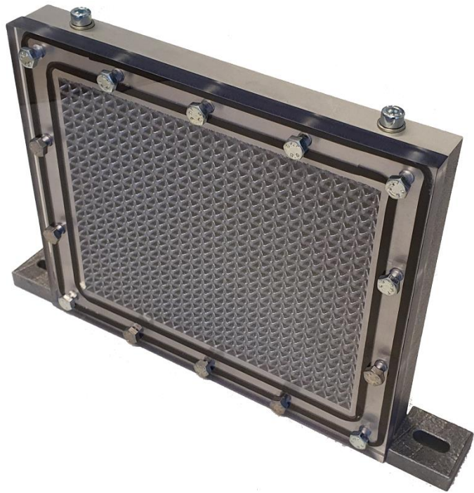
Figure 6.14: ITS specimen open wall window without any MLI cover, in order to verify the macroscopic PCM melting behaviour and the melting fronts by optical (visible and IR) recordings of a large-scale flat plate with integrated lattice
