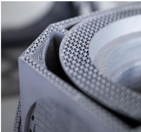
Figure 3.2: ITS demonstrator exhibit variant without completed additive print job, to visualize the ITS double wall design with integrated lattice structure [FHA-21]
