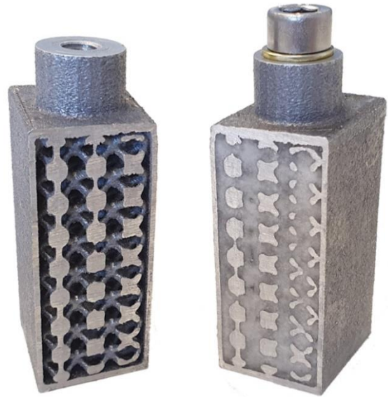
Figure 3.1: The specimen sectional view illustrates the monolithic double wall ITS integral design, where lattice matrix is integrated and PCM is embedded in the void as macro-encapsulation (left: without PCM, right: PCM infused) [WIL-21]
