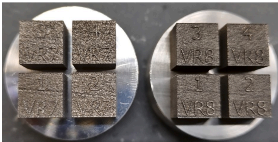
Fig. 8. PBF-LB fabricated 10 \times 10 \times 10 \text{ mm}^3 cubes of pure matrix material AlSi7Mg0.6 (left) and the composite AlSi7Mg0.6 + 1 wt.% TiCnm made with the 15-min-mixed blend (right).
