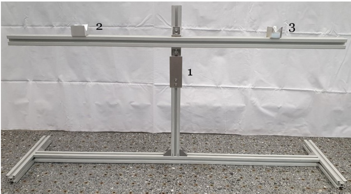
Figure 3.9 Mounting system with supports of the isostatic mount
