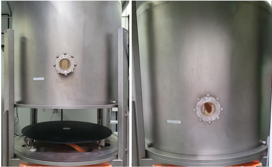
Figure B.2 TVC with bell opened (left) and closed (right)
