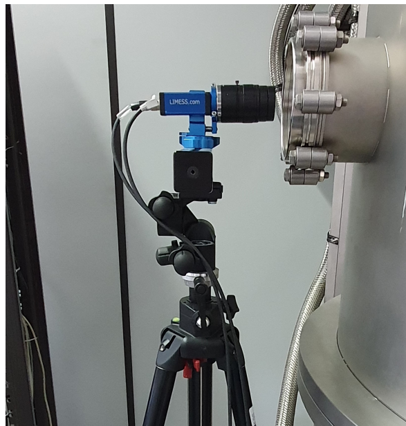
Figure 3.11 DIC system in leveled condition on tripod
