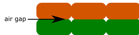
Fig. 2 Schematic section through the printed object with two layers printed in the same direction
