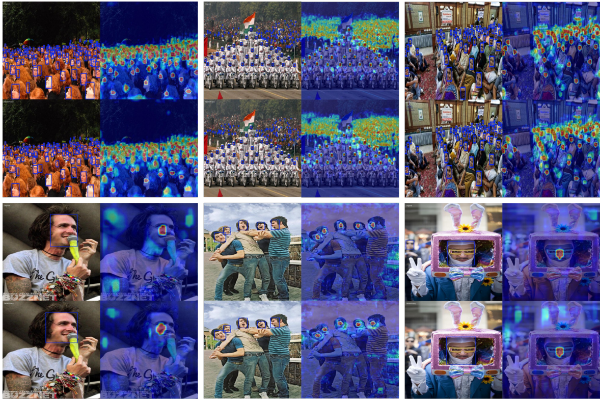
Figure 4.29: The top images in each set show the face bounding box predictions made by YOLOv8 large, trained on the original data (left). The corresponding class activation map (right) uses a red-to-blue color scale, with red indicating areas of highest influence on the model’s prediction. For large faces, a relatively small area is used to make the decision. The bottom images show the same results for the model trained on anonymized data. All images are from the original validation split of WIDER FACE (see Section 3.2.1), only training data is anonymized.
