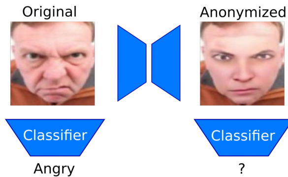
Figure 3.7: To evaluate utility retention, the images of a dataset labeled with expressions are anonymized with different de-identification approaches. Then, the accuracy of a machine learning-based expression classification model is calculated. The higher the accuracy after anonymization, the better the utility retention.
