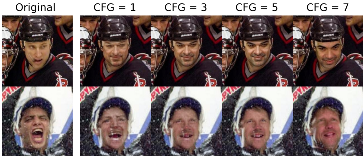
Figure 4.22: Example images from the LFW dataset (see Section 3.2.1) anonymized with StablePrivacy. The higher the CFG (guidance) scale, the more closely the Stable Diffusion model follows the image prompt during inpainting. Facial features such as the thickness of the lips and the shape of the nose resemble the source more closely for higher values of the CFG scale. At the same time, pose and expression also align more closely with the image prompt, potentially reducing the diversity of anonymized training datasets.
