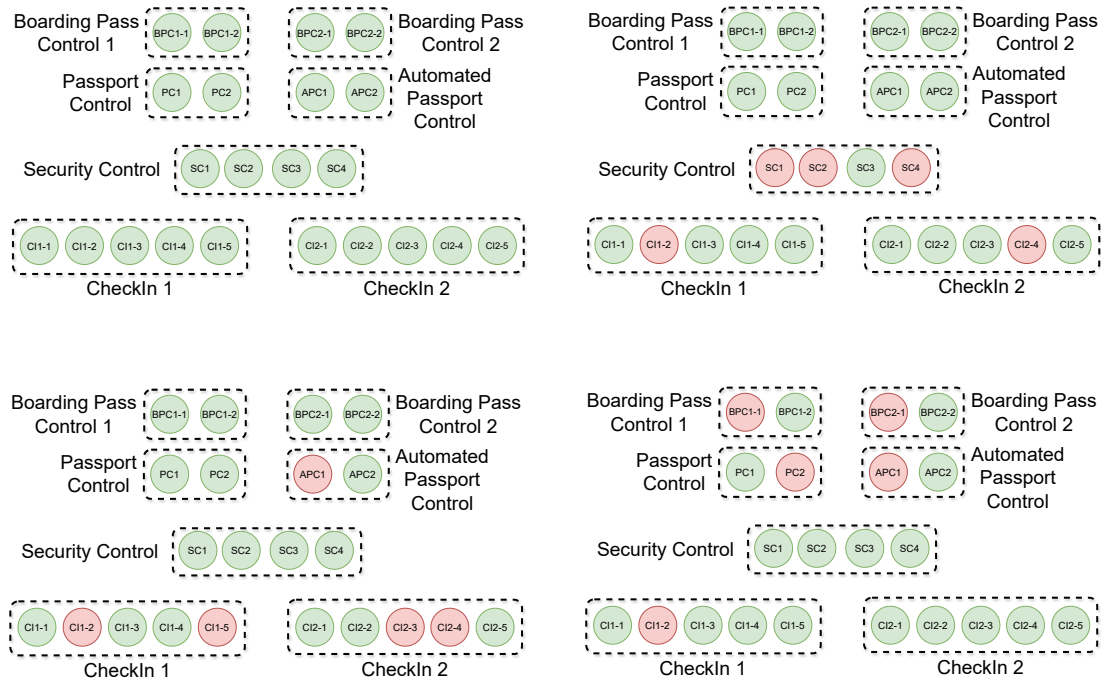
Figure 5.12: Based on the layout given in Figure 5.9 the four used scenarios are displayed (initial state: top left; scenario 1: top right; scenario 2: bottom left; scenario 3: bottom right). While all scenarios, except the initial state scenario contain a cumulative number of five malfunctioning devices (indicated in red), the devices are distributed differently over the process groups. (Koch et al., 2019a, ©IEEE 2019)
