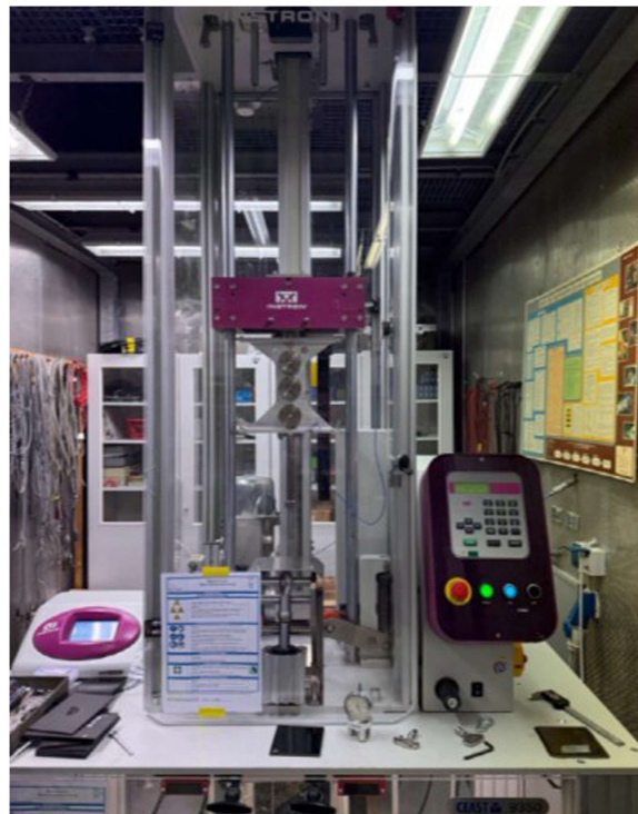
Figure 2. Drop tower setup—Instron 9400.
