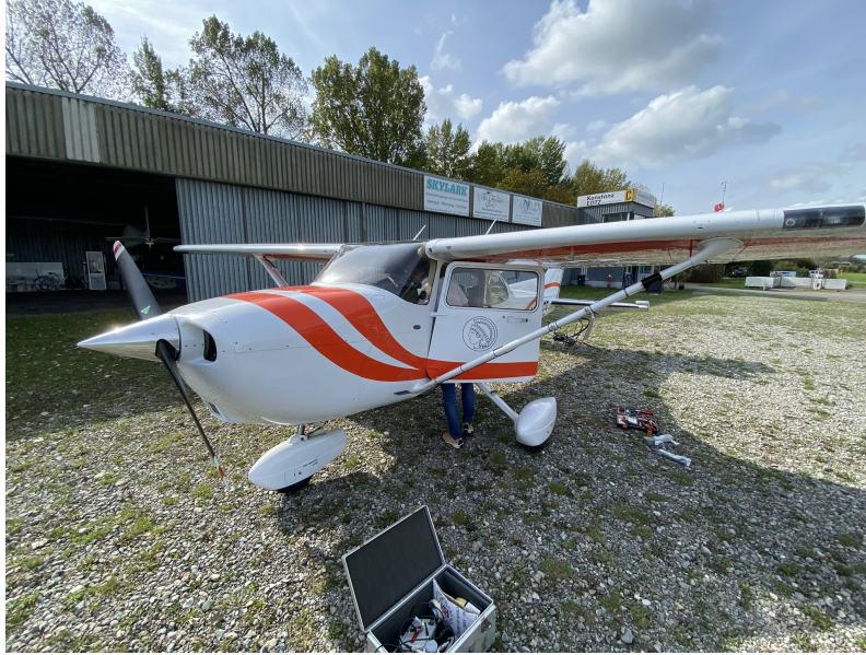
Figure 57: Assembly of external measurement equipment on a Cessa 172 wing structure.
