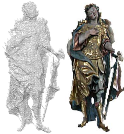
Fig. 7.13 Create textured triangular meshes (13846 faces occupying 1.66 MB)
