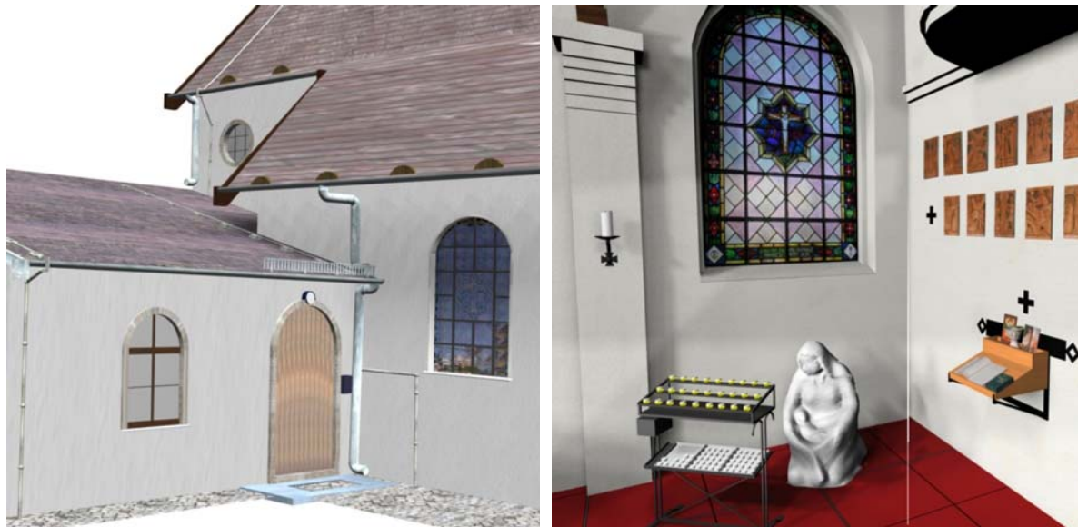
Fig. 7.23 Detailed views over the exterior and interior of the church from the campus of the University of Bundeswehr Munich (see Fig. 3.6 for thermographic representation). The images (1160x1080) are rendered using default Scanline render in 3ds Max 6 (render time approx 15 seconds)
