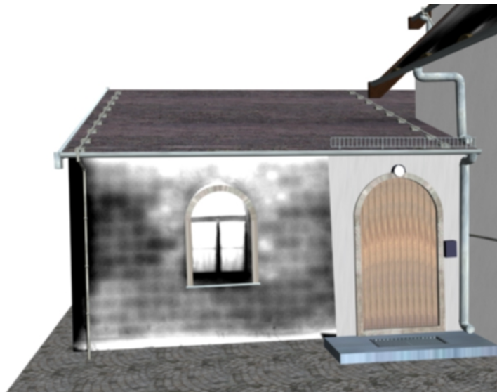
Fig. 3.6 Building 3D model mapped with thermographic and digital images (see Chap. 7.4)
