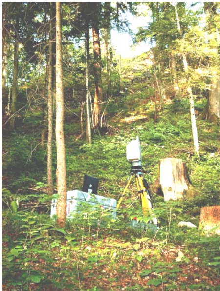
Fig. 7.25 Laser scanner HDS 3000 mounted at one of the scanning positions to acquire data needed in DGM creation (the large vegetation coverage can be observed)
