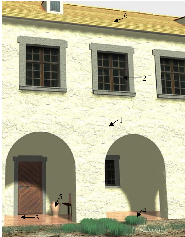
Fig. 5.10 Generic materials in a VR (virtual reality) scene using 3ds Max 6 (see project “Hohenburg”, Chap. 7.5); for a description of the used terms see Annex VII
