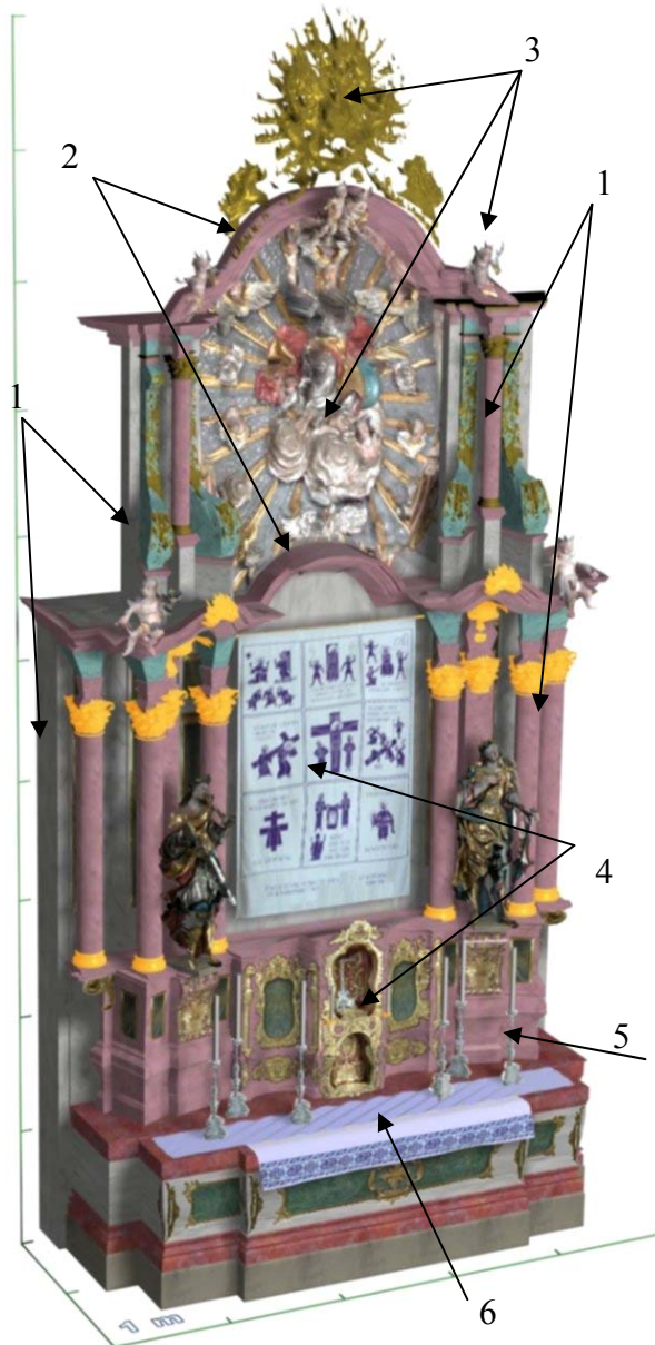
Fig. 7.17 Main altar – St. Michael church (default 3ds Max Scanline renderer). The numbers are identifying the above mentioned methods used to create the highlighted objects. The model contains approx 200000 faces and 40 materials (approx. 15 MB in *.max format).
