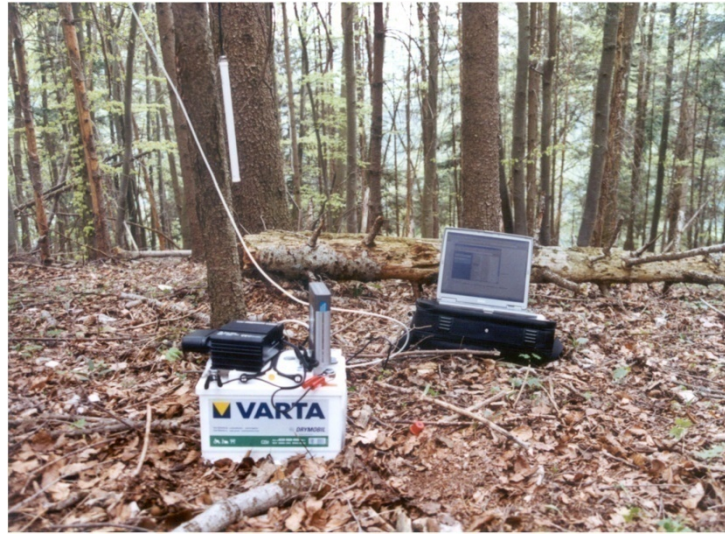
Figure 79: Field Geoserver and WLAN Router
