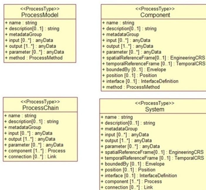
Figure 11: SensorML Conceptual Models [OGC-SensorML, 2007]
