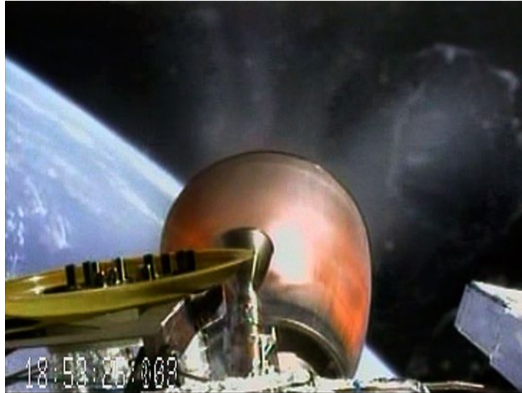
Figure 2: Radiation cooled Merlin upper stage rocket motor on a Falcon 9 test flight [9]
