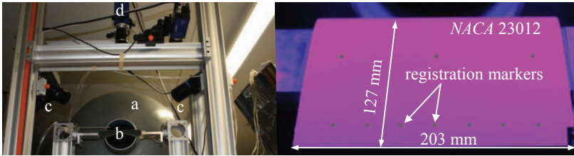
Fig. 5.5.: Experimental setup at the open-jet wind tunnel (a) for the low-speed PSP validation experiments on a NACA 23012 airfoil (b); 405 nm LED excitation (c) and camera with signal filter (d), from Bitter and Kähler (2011).
