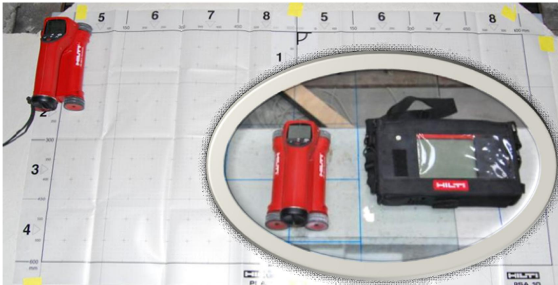
Figure C-3: HILTI Ferros scanner PS200
