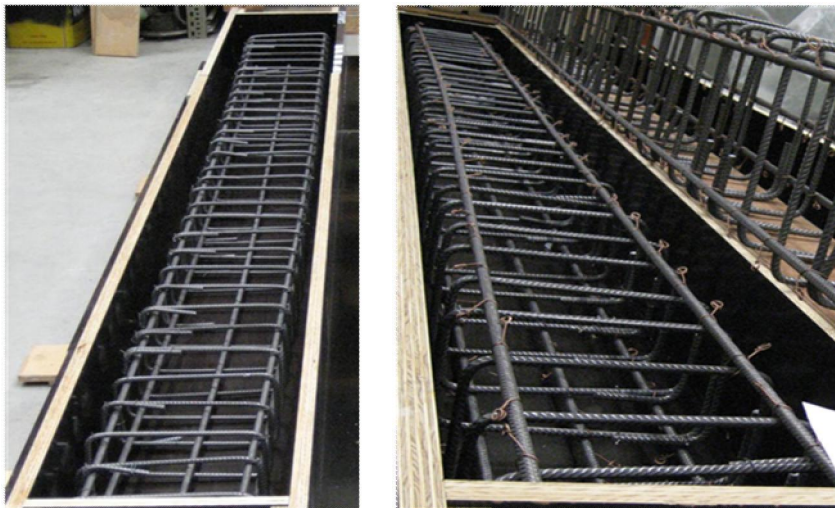
Figure D-6: Formwork and reinforcement of test specimens in Series-2
