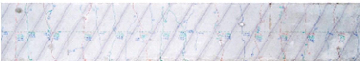
N6w3, loading 56kN, 56 % of Ultimate load
