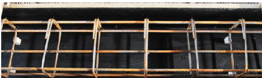
Figure D-4 Formwork and reinforcement of test specimens in Series-1 (a)
