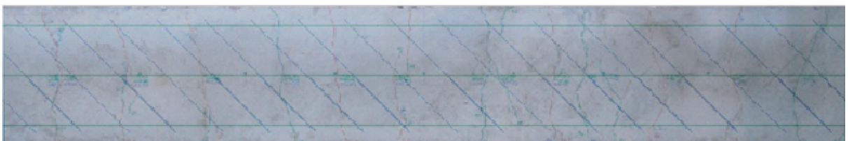
N5w3, loading 50kN, 69 % of Ultimate load
