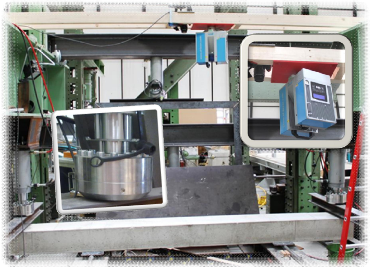
Figure C-4: Measurement instruments with digital camera and Laserscanner
