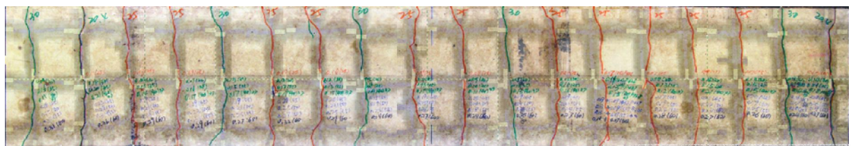
Ac1, load 60kN, 79.1% of Ultimate load
