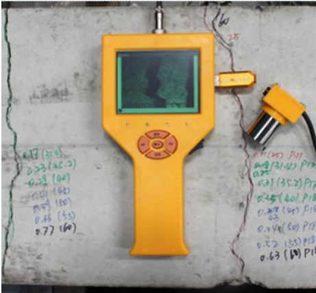
Figure C-5: Crack width measurement instrument PTS-C10
