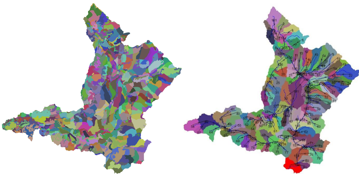
Figure 7.9 Hydrotope and routing structure developed during preprocessing of SWIM at Gibe III catchment
