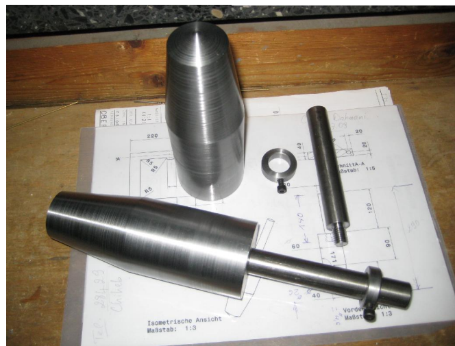
Figure 18: Constructed experimental electromagnet, with its exchangeable tip system (bottom) and after assembly (top). The top left figure shows the magnet after galvanization and featuring a temperature measurement strip.
