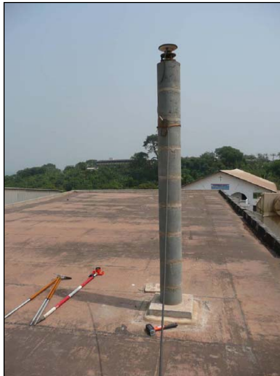
Figure 5-14: Show the monument located at the Takoradi Regional Survey Office as part of the GRN
