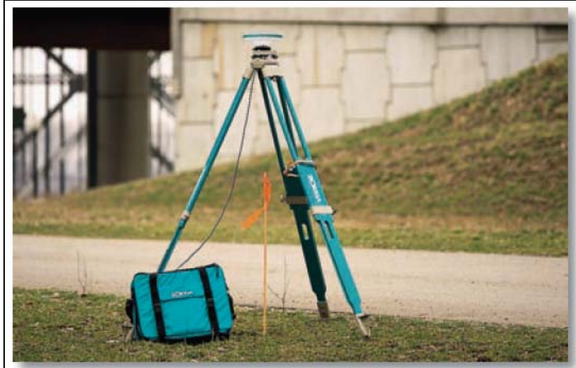
Figure 5-16: Picture of an antenna SOK702 used for the data collection mounted on a tripod
