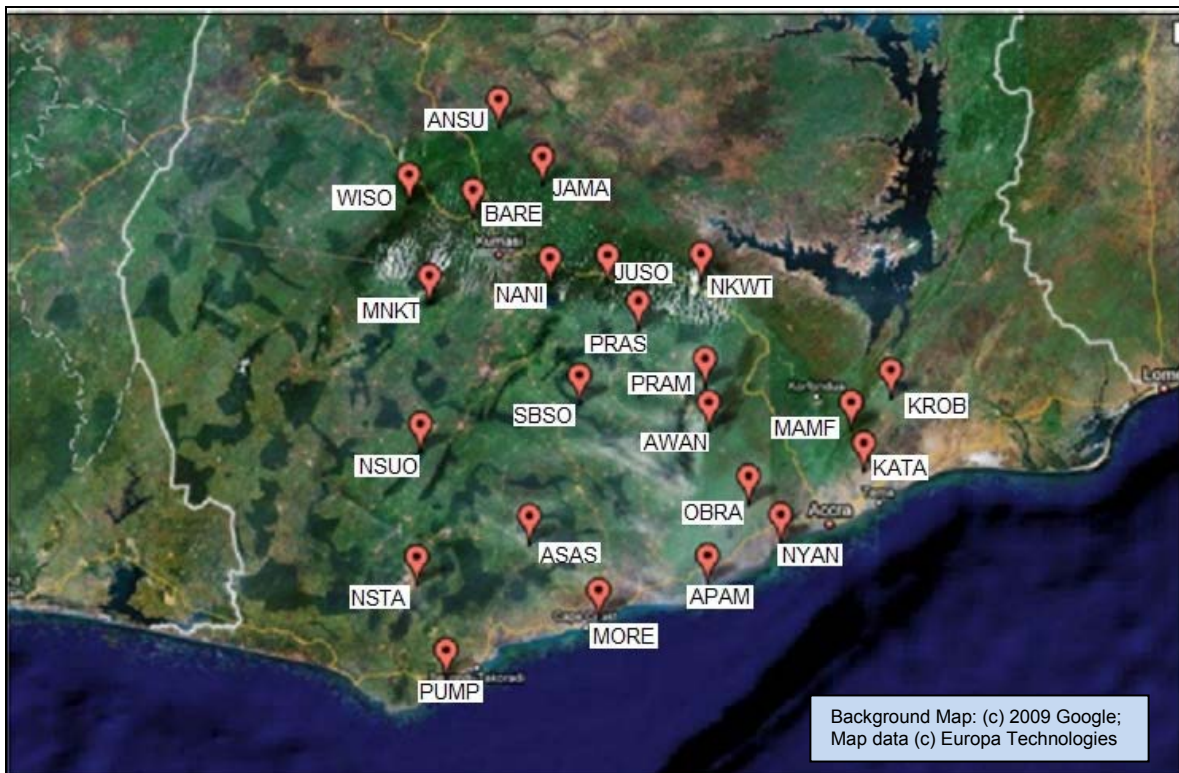
Figure 8-1: Showing the locations of the Trig Points for the determination of Transformation Parameters
